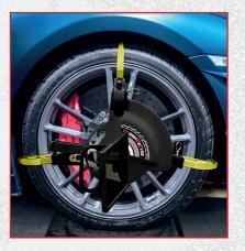
The special feature of the new ClampOnTyre clamp is that it does not touch the rim, but it grips the tyre by means of three shaped hooks as shown in the figure below.
