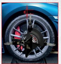
For a typical installation of the product, the "d" distance between the tyre and the wheel arch should be at least 30 mm.
